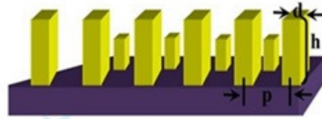
Fig.7: (b) Schematic of the substrate showing the inter-columnar distance
